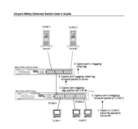
In the above example, step 4 is the key element. Because the packet has 802.1Q VLAN data encoded in it's header, the ingress port can make VLAN-based decisions about its delivery – whether server #2 is attached to a port that is a member of VLAN 2 and thus should the packet be delivered, the queuing priority to give to the packet, etc. It can also perform these functions for VLAN 1 packets as well, and in fact, for any tagged packet it receives regardless of the VLAN number.
